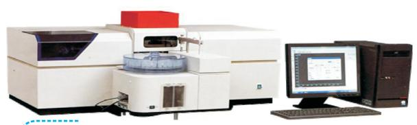
The atomic absorption spectrophotometer is an inorganic analysis instrument. It can be widely used in the quantitative analysis of the microelements and trace elements in the metallurgical, geologic, oil, chemical, medicine and health, industrial, farming and forestry, commodity inspection and environmental protection fields, etc. It can determine more than 70 elements.
