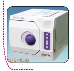
According to EN13060 standard completely. Manual door locking system. Sterilization temperature: 121, 134 Cent degrees. Programs: 10 programs(Including test programs). Test program; Helix test, B&D test, Vacuum test. Drying Program: Vacuum drying. LCD display. Sterilization record: mini external printer is available. Safety: safety valve, temperature control, pressure protection
