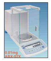
Balance accuracy is guaranteed by automatic internal calibration dependant on time and temperature changes.
